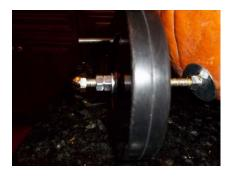
\*\*The purpose of the acorn nut is simply to protect you from scratches or cuts from the threaded rod. A small piece of duct tape or something similar will do the trick at less expense.
