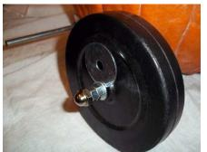
Place one wrench over one hex nut and the other wrench over the second hex nut. Rotate one hex nut to the right and the other to the left. This will give you a tight joint that you will not be able to move by hand.
