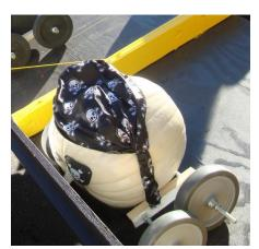
Note the outboard stabilizer bar attached to the axle.
