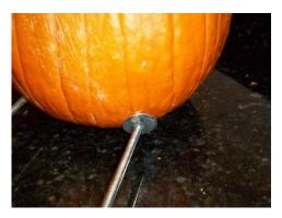
HELPFUL TIP: After repeated use, axles may bend or warp, especially if your racer has crashed. Do a check of the axles before each race to make sure they are straight.
