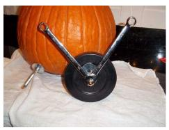
To create the LOCK NUT, simply rotate two hex nuts onto each other. For this step, you will use the two ½ inch wrenches. You will have EIGHT points on the four axles where you will need to make LOCK NUTS; one on each side of each wheel.
